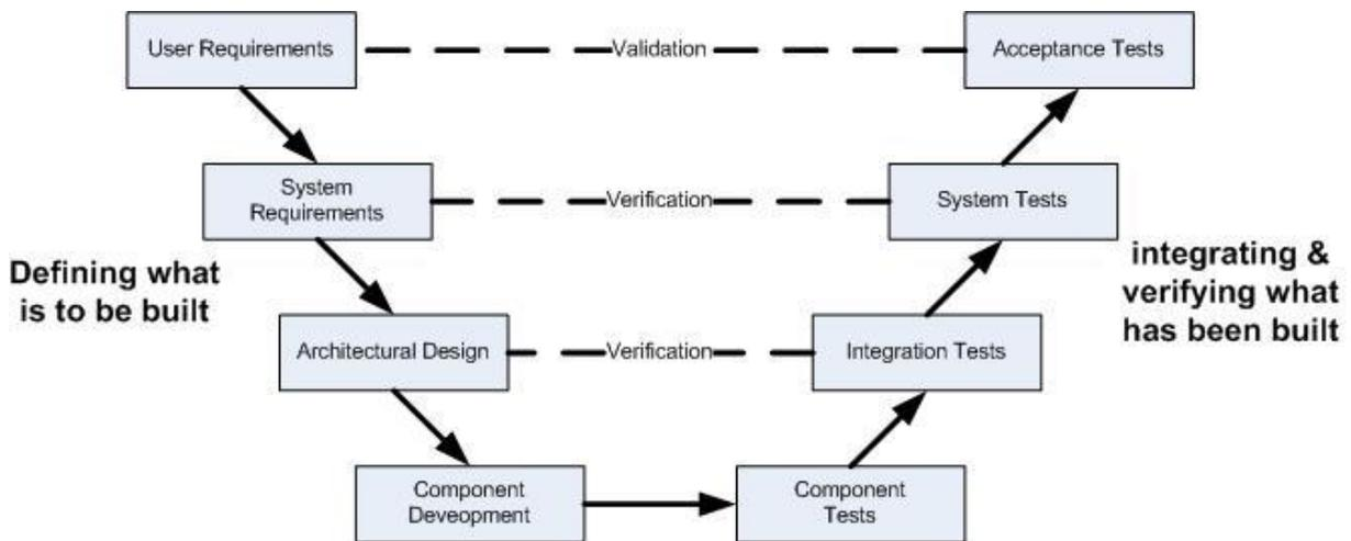
**Figure 5-3: V-diagram form of systems engineering life cycle.**
