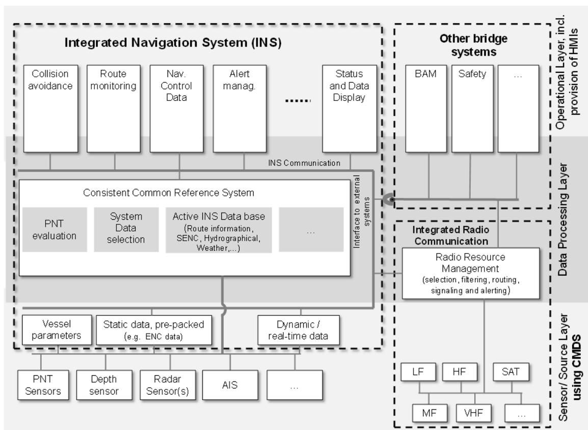
**Figure 3-2: Generic technical shipboard architecture supporting e-Navigation**
