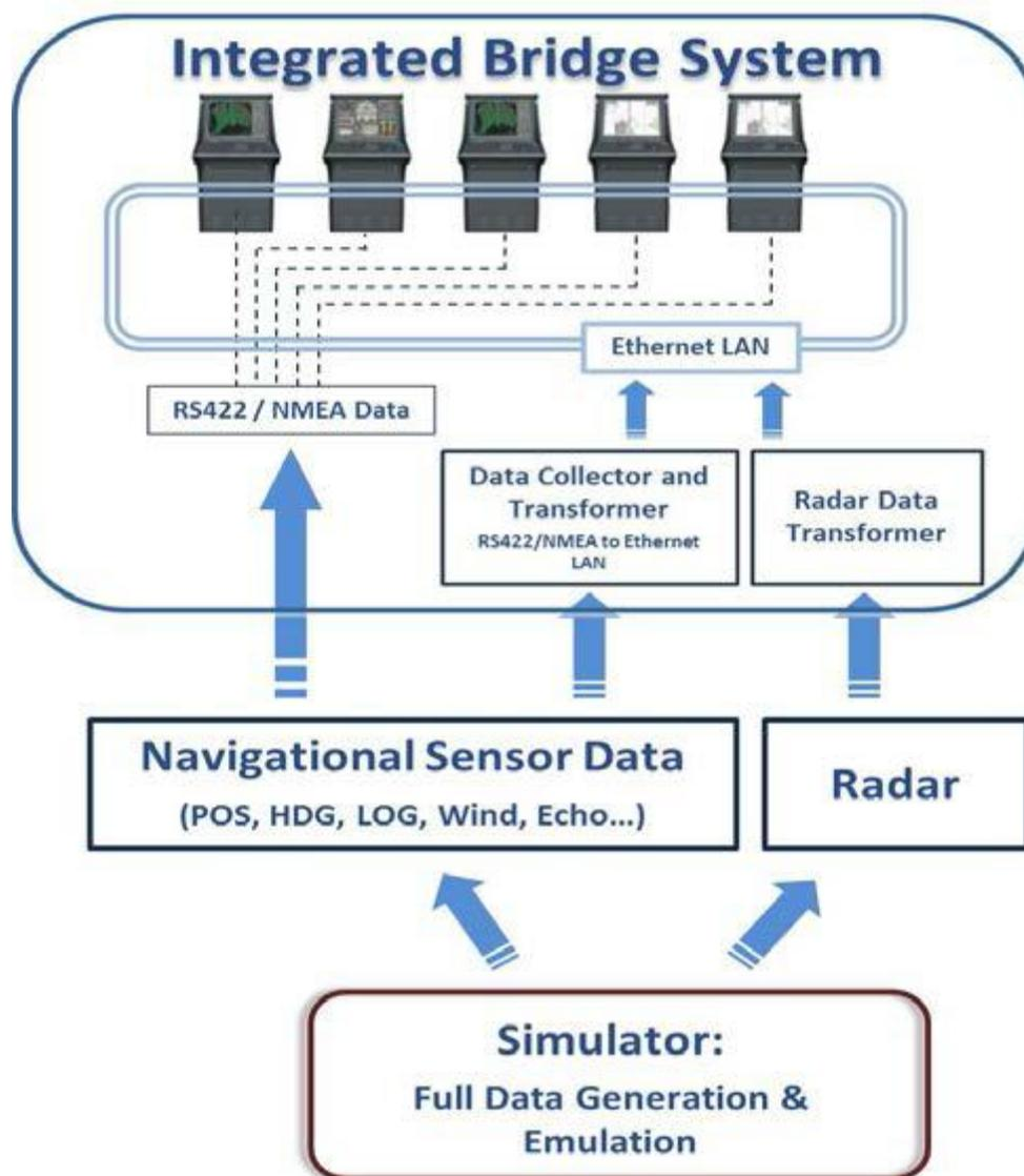
**Figure 5-6: IBS data flow structure**
