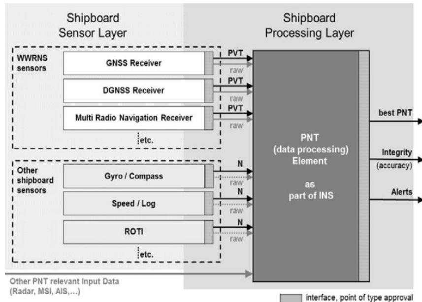
There are sensors for each data source which feeds the data it receives into the processor. The processor uses an algorithm to make a decision on what is the source of PNT with the most integrity; it then makes a decision of how to do to inform the mariner.
