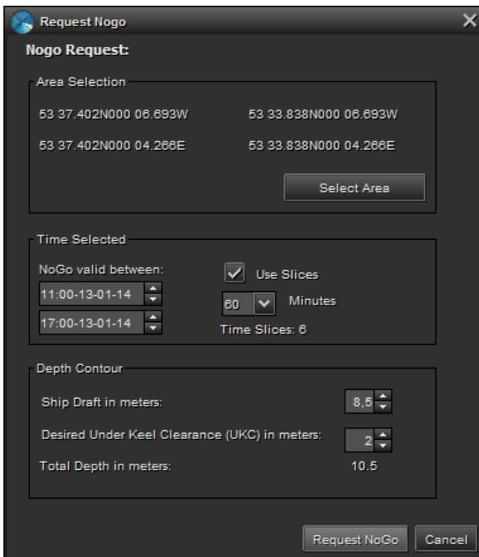
Figure 4: Vessel selects area by drawing corners on chart and input time interval, ships draft and desired UKC. Choose to use time slices for every 60 minutes in interval.
