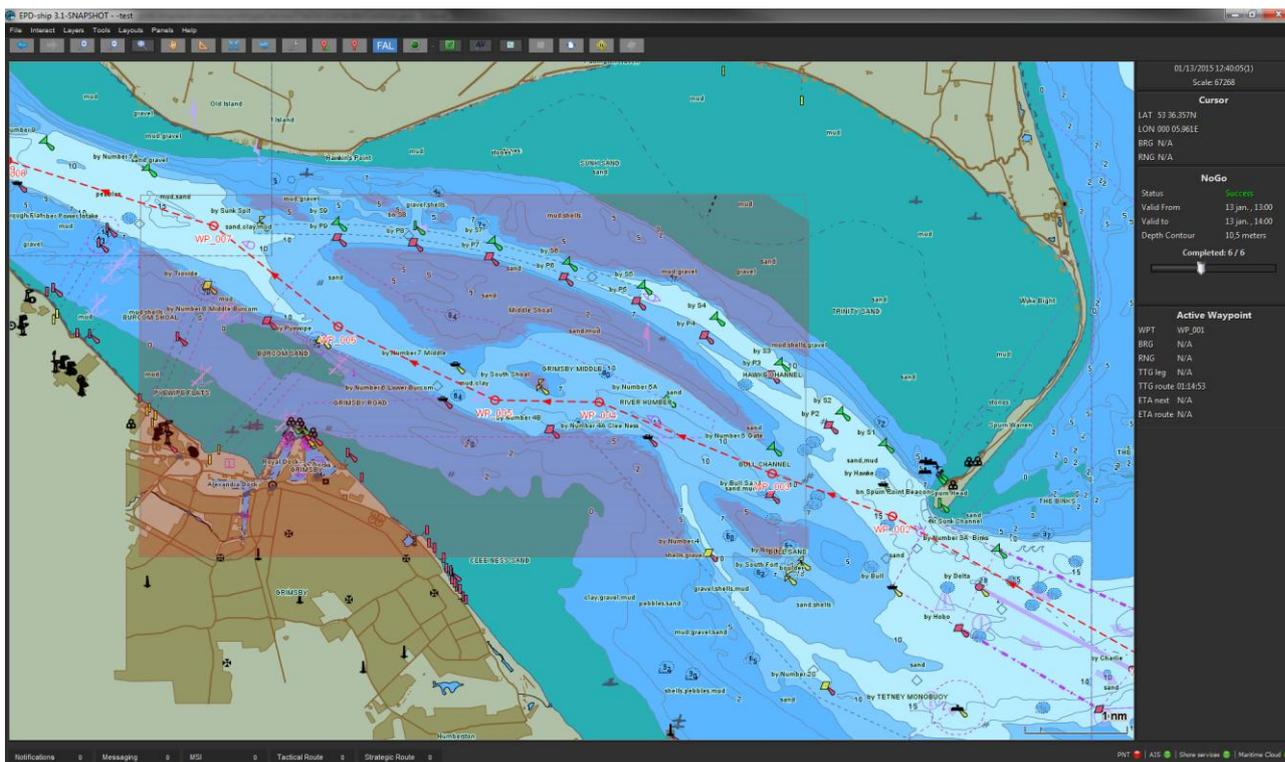
Figure 6: From 13:00 to 14:00 southern channel opens as water rises. With the time slices it is possible to browse through time and easily see the changing water level and when channels or areas are navigable for vessel.
