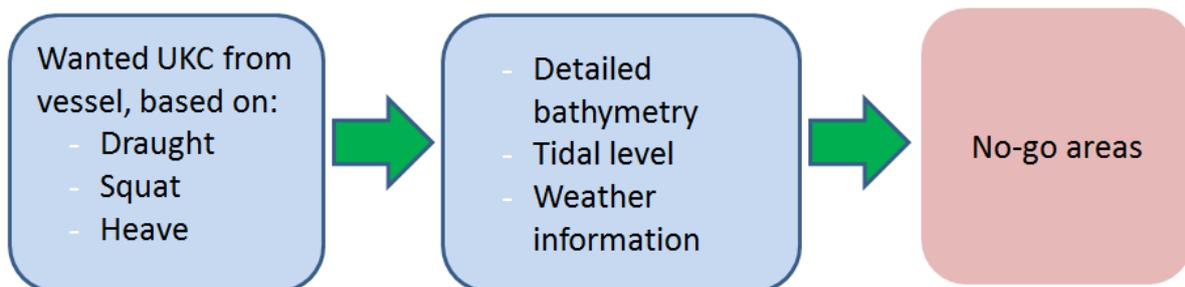
**Figure 1: The diagram shows parameters needed to calculate the UKC advice. (Source: Porathe, 2006)**
