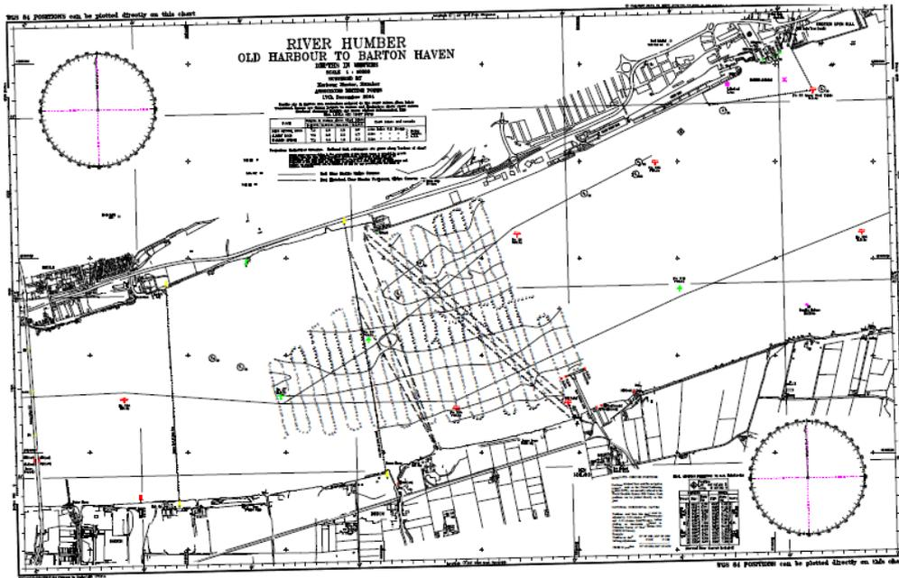
**Figure 9: Example of a new survey map from the Humber River. The format is a paper map scanned into a pdf file. The track of the survey vessel can be seen in the middle of the image. The survey track consists of depth figures. (Source [www.humber.com](http://www.humber.com))**
