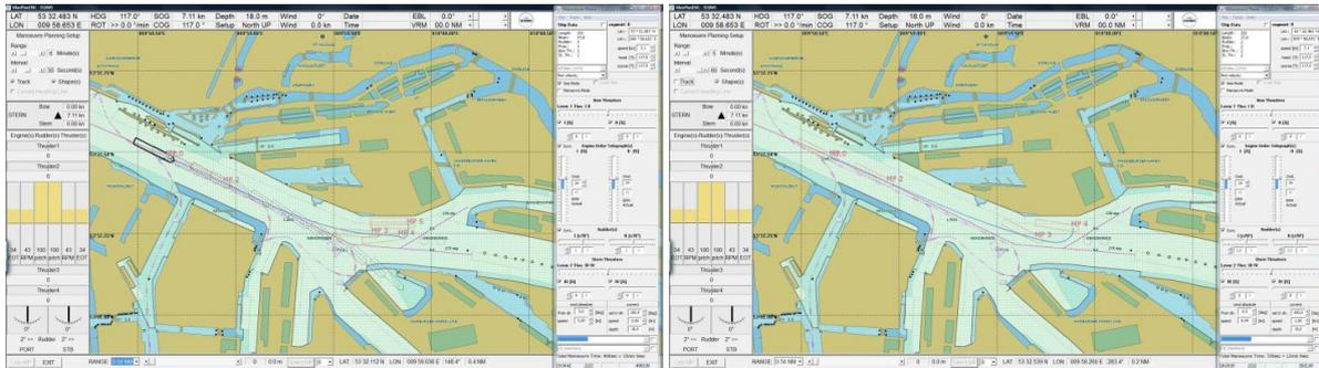
**Figure 13:** Alternative Manoeuvring plans – Left: with Total Manoeuvring Time 15 min more efficient because of immediate transfer to crabbing. Right: with Total Manoeuvring Time 12 min - Most efficient because of using the supportive effect of current for crabbing
