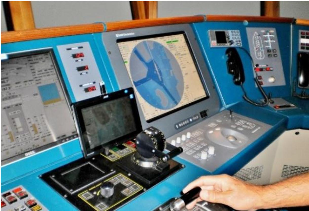
**Figure 15:** Portable Setup for Prediction Display on ECDIS in Monitoring Tool on Students Laptop on a Full-Mission Bridge of a Ship handling Simulator– the prediction is controlled by the Bridge Handle. The dynamic prediction shows the future manoeuvring track whereas on the Radar Screen the static path prediction shows still a straight line according to the initial conditions of the ship
