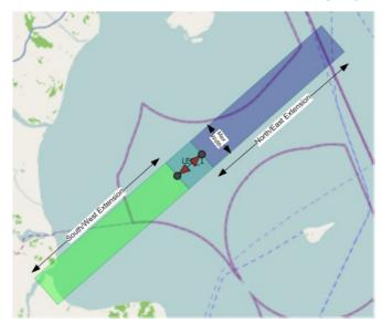
The Maximum Extension is used to control drifting groundings and area collisions, i.e. drifting groundings and area collsions will only occur within the indicated boundaries. You can use 'Settings/Project Settings...' to modify Widths/Extentions for all Legs and/or set the default value for new Legs.
