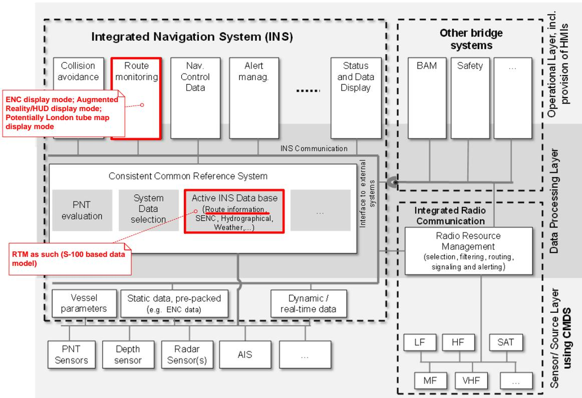
**Figure 3-9: Mapping of the RTM to the generic shipboard architecture**
