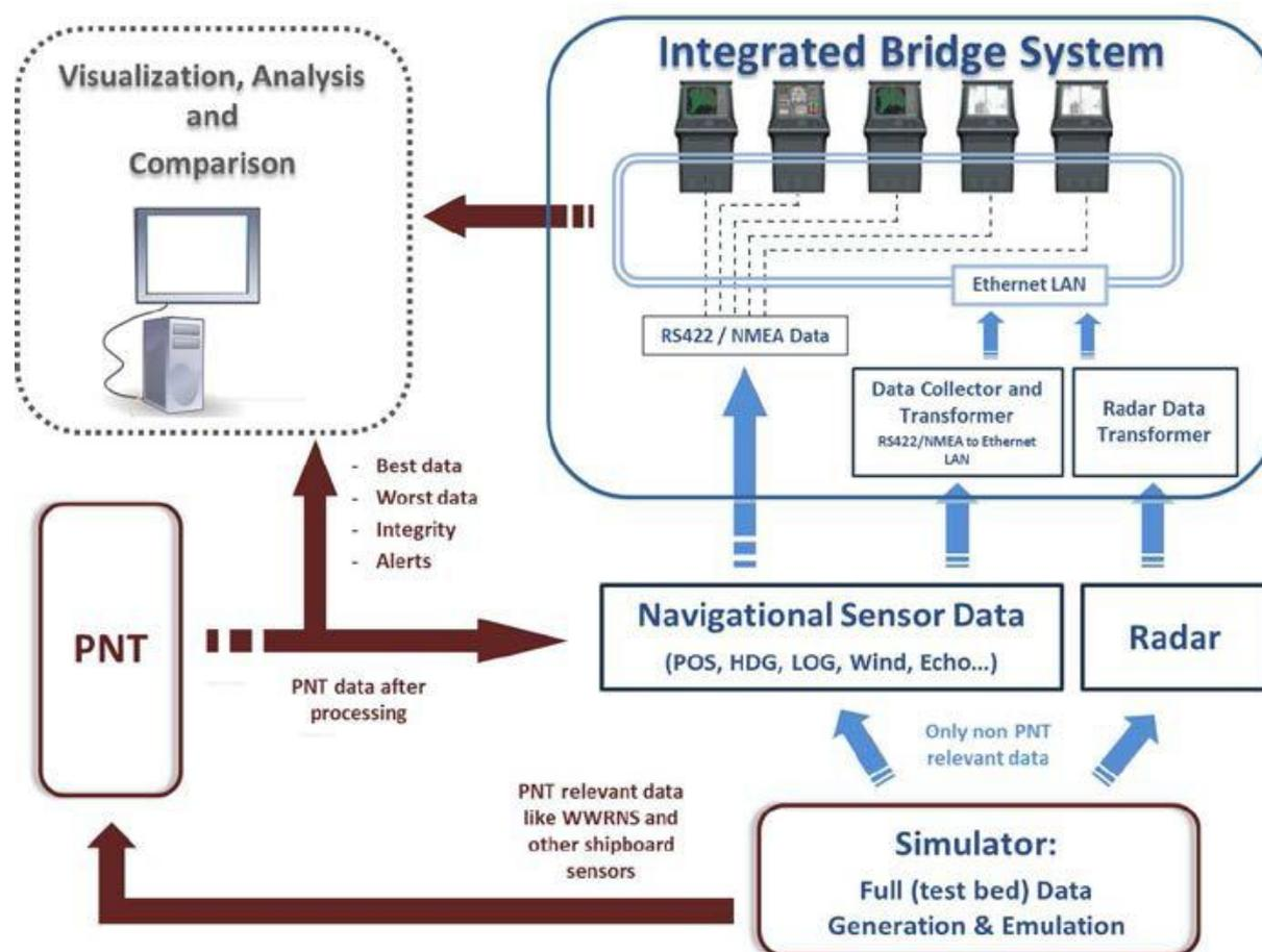
Figure 5-7: Data flow architecture for Resilient PNT tests
