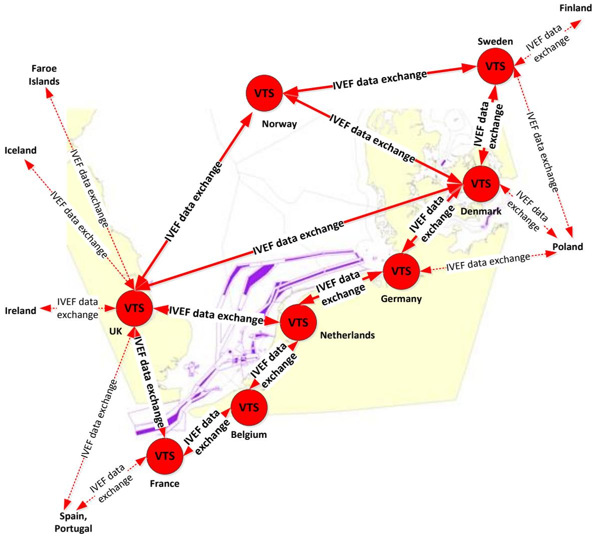
**Figure 3-21: Topology of a potential future IVEF-based real-time, highly reliable network for real-time, highly reliable, integrity-assured and/or validated vessel track data stream exchange amongst VTS stakeholders in the NSR – the ‘NSR VTS Handover Network’**
