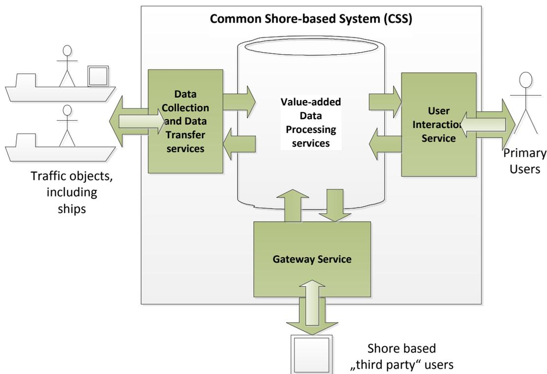
**Figure 3-3: Structural overview on Common Shore-based System Architecture (CSSA) in its context**
