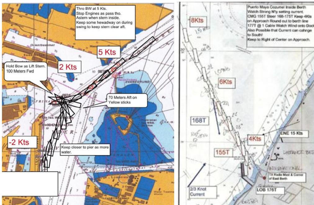
Figure 8: Samples of two plans for berthing a ship in a harbour
