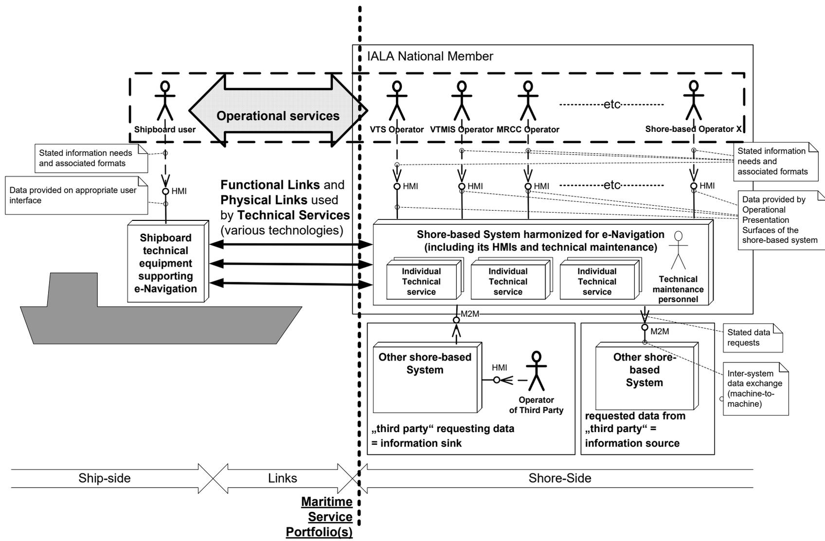
Figure 3 The overarching architecture with focus on the shore-side (simplified representation; i.e. without CMDs and WWRNS)
