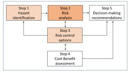
IWRAP supports steps 1 (to some extent), 2 and 3 (to some extent) of the FSA process. The hazards that can be identified are groundings, allisions and collisions. The calculated likelihood of those accidents can be differentiated by ship type and ship size class and be presented as a "heat map" on top of an ENC or chart Bitmap.
