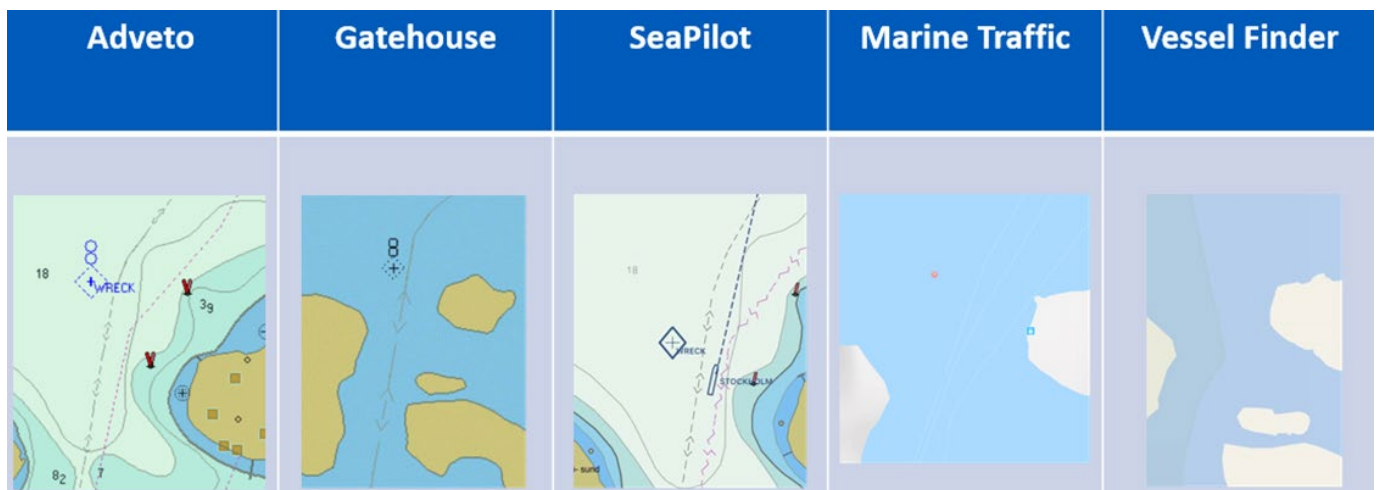
Figure 2 Variation of imagery due to software and type of ECDIS equipment or mobile application
