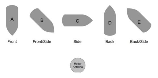
Figure 25 Target aspect angle relative to the radar antenna
