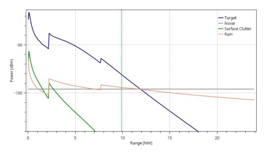
Figure 6 Example of received power versus range
