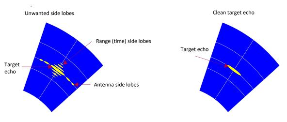
Figure 12 Range and antenna (azimuth) side lobe effects
