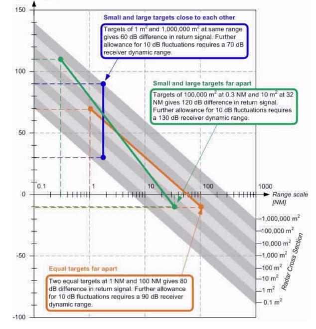
Figure 11 Dynamic characteristics of the signal received versus target RCS and target range
