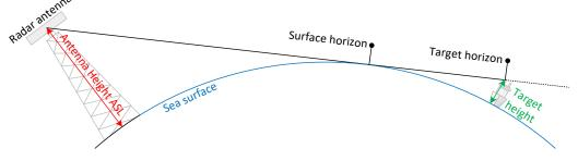
Geometry, antenna height and target height Figure 5
