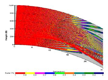
Figure 15 Coverage diagram, elevated duct
