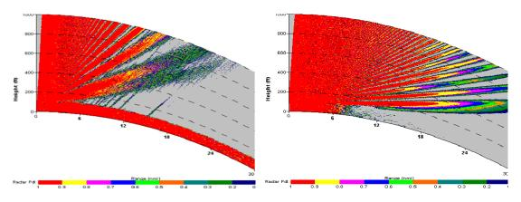
Figure 16 Coverage diagram based on a measured condition
