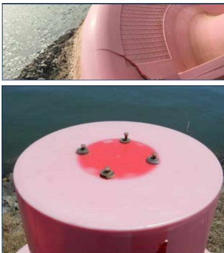
***Figure 5 Plastic buoys in Abu Dhabi/UAE–The effect of extreme sun light (UV) on the materials***
