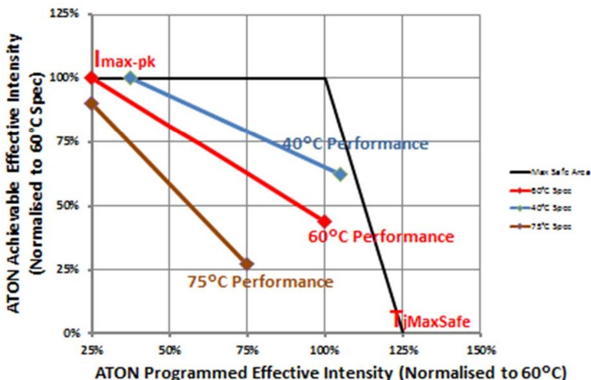
**Figure 9** *AtoN performance limits vs combined ambient temperature*
