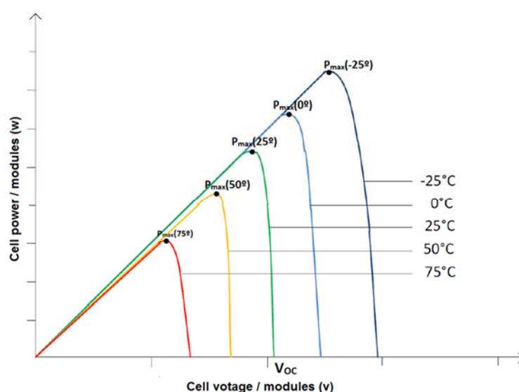
**Figure 6** *Impact of temperature in the power of a solar panel*
