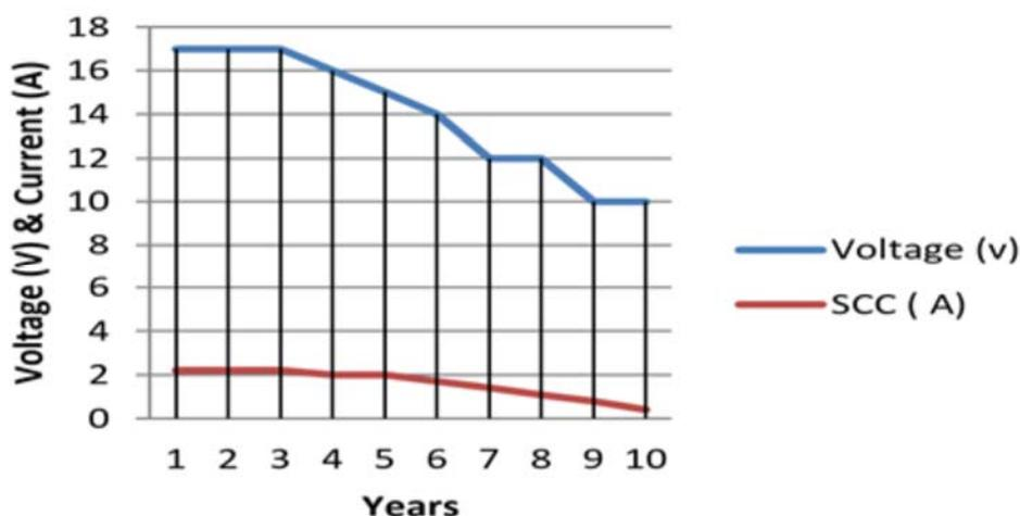
**Figure 8** *Power reduction over time of a solar panel deployed in an extreme heat environment*
