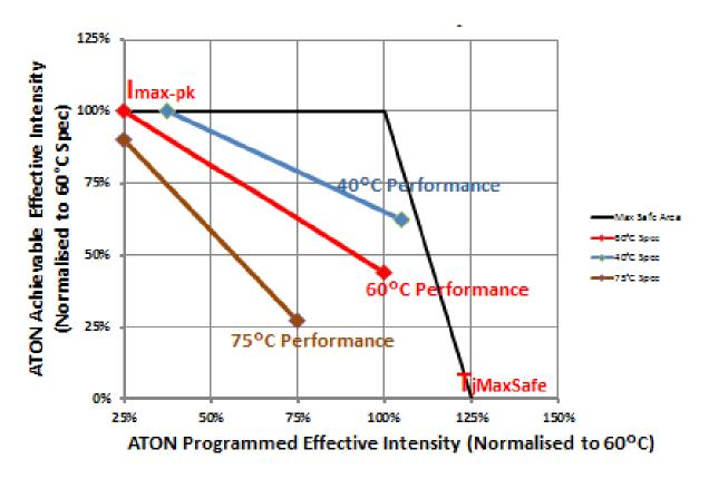
Figure 9 AtoN performance limits vs combined ambient temperature
