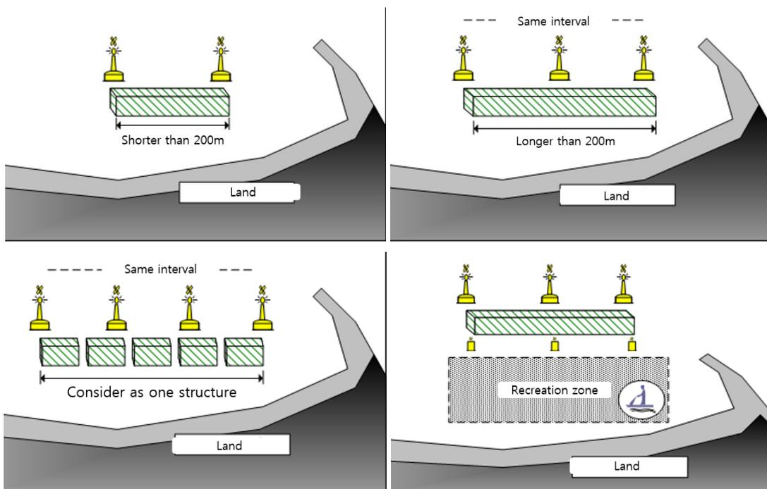
Figure 6 Examples of marking breakwaters with floating AtoN
