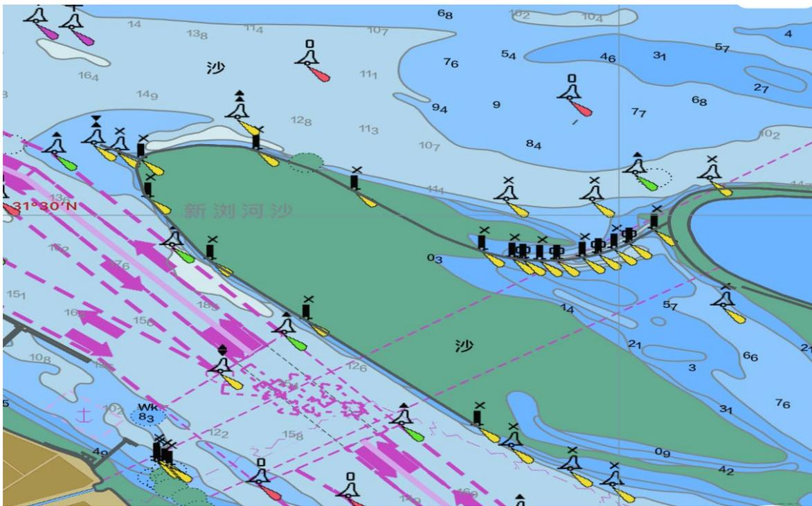
Figure 4 New Liuhe sand bar and Nanshatou Channel submerged breakwater (dikes), Yangtze River Estuary, China
