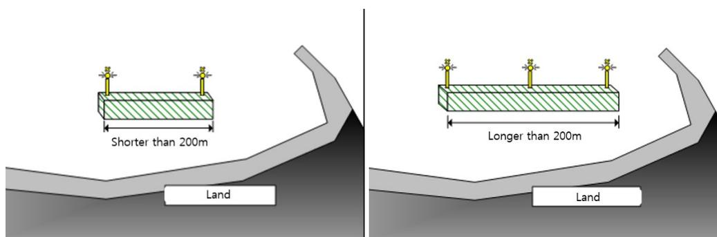
Figure 5 Example of marking breakwaters with fixed AtoN
