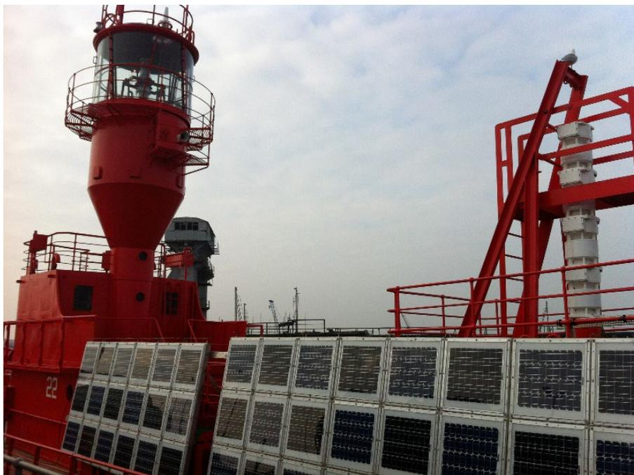
*Figure 22 An example of a solar array on a lightvessel*
