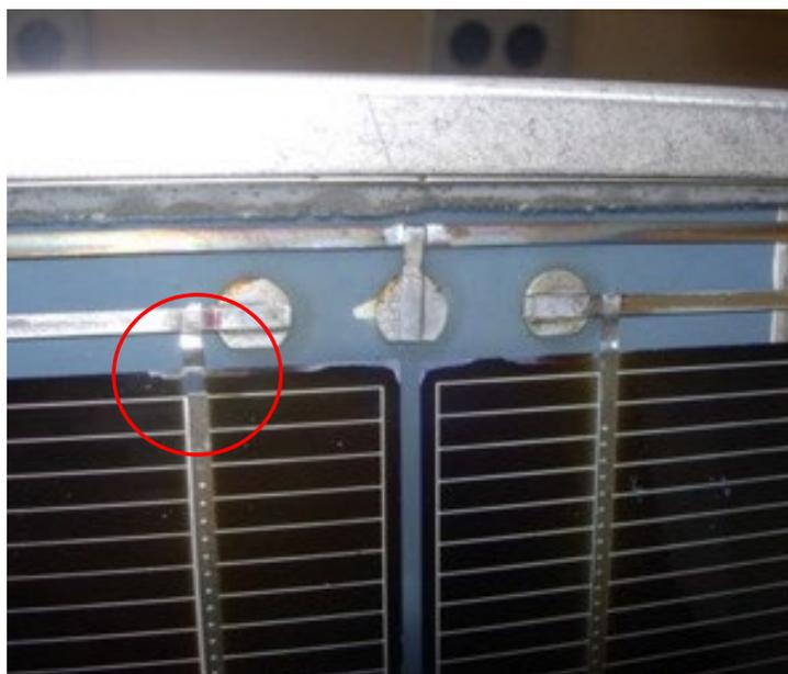
Figure 30 Ribbon fracture.
