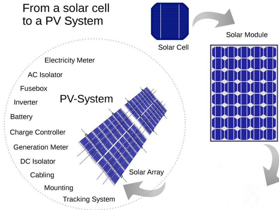
Figure 1 Component of a solar system by Rfassbind - Own work, Public Domain,
