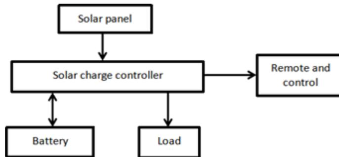
Figure 12 Solar charging system with a controller
