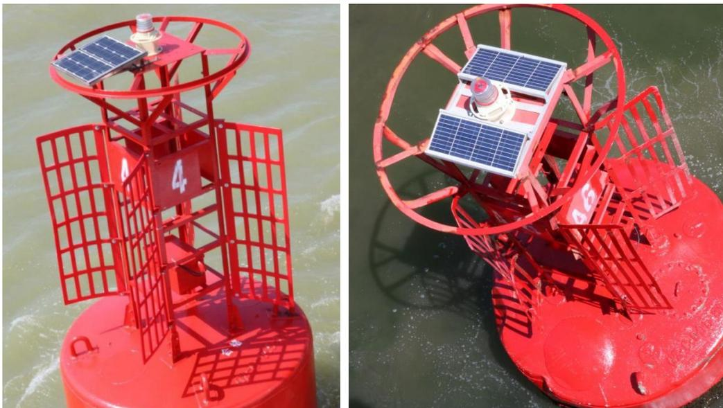
*Figure 24 Wind impact to solar modules on buoys*
