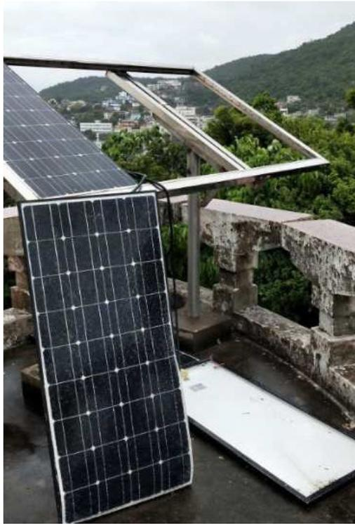
*Figure 23 Example from China of damaged solar modules following a super typhoon*
