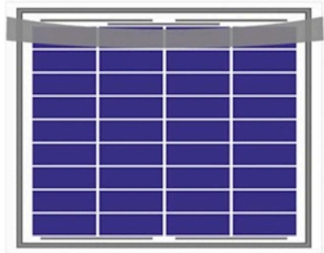
The above example of shadowing could result in a 90% reduction in power output.
