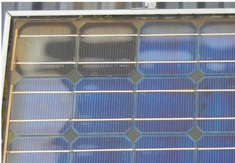
*Figure 35 Encapsulant discolouration*
