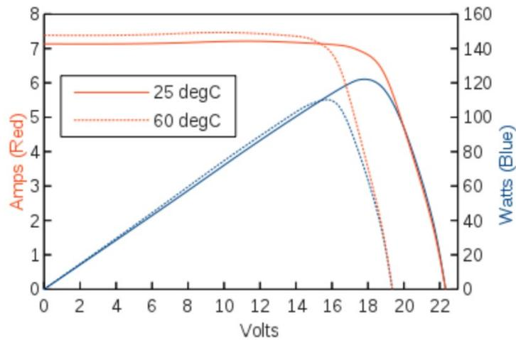
Figure 14 Impact of temperature on solar module performance
