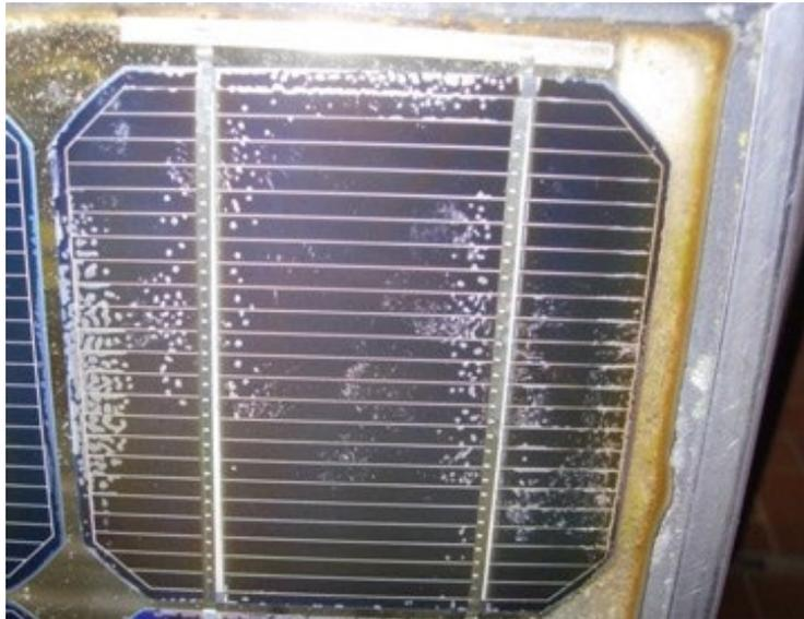
Figure 31 Cell corrosion.
