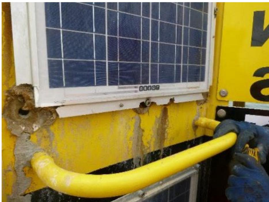
*Figure 36 Impact of leakage current*
