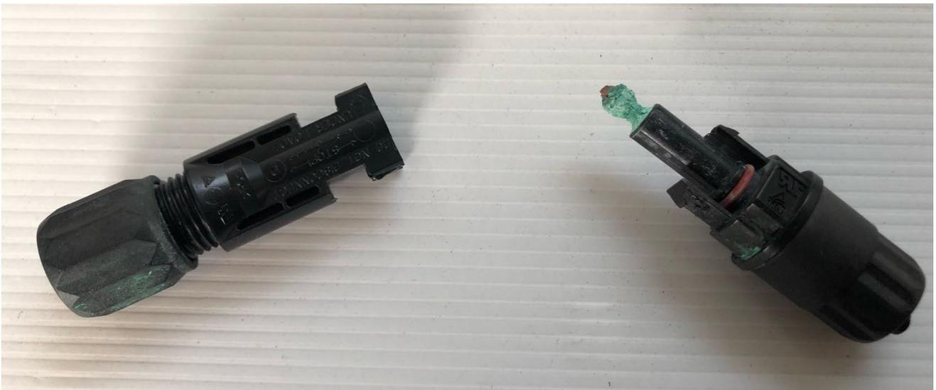
Figure 40 Connector failure
