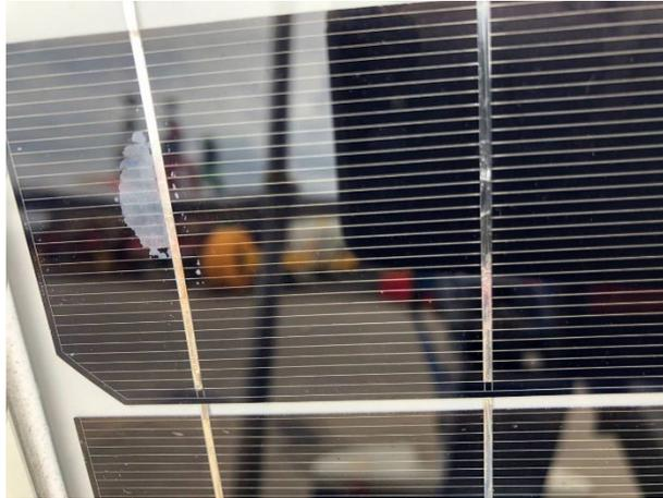
Figure 39 Delamination on a new solar module
