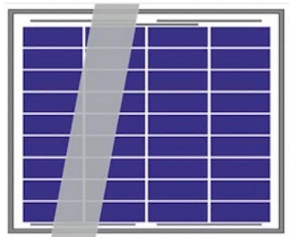
The above example of shadowing could result in a 75% reduction in power output.
