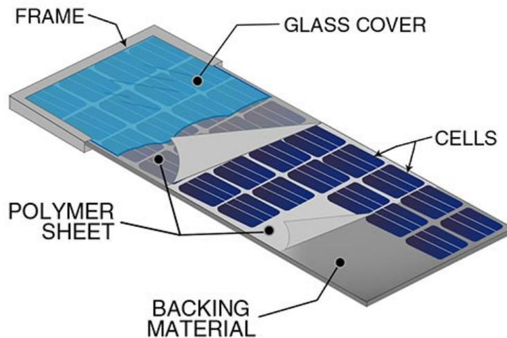
Figure 9 Figure showing the construction of a solar module from [www.sunnetsolar.com](http://www.sunnetsolar.com)
