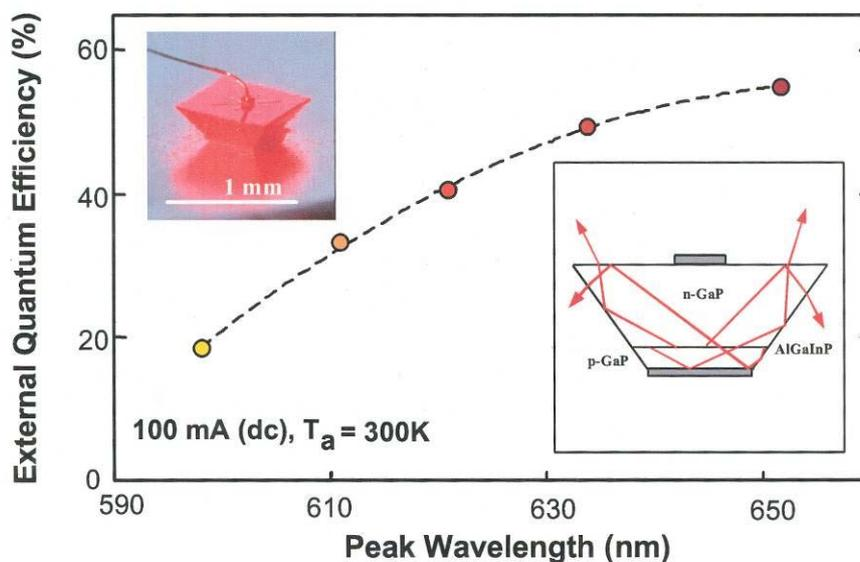
**Figure 6** *AlInGaP/GaP Truncated-Inverted-Pyramid (TIP) Die*
