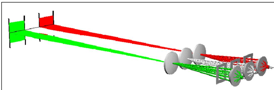
***Figure 14*** Beam arrangement for 3 projectors
