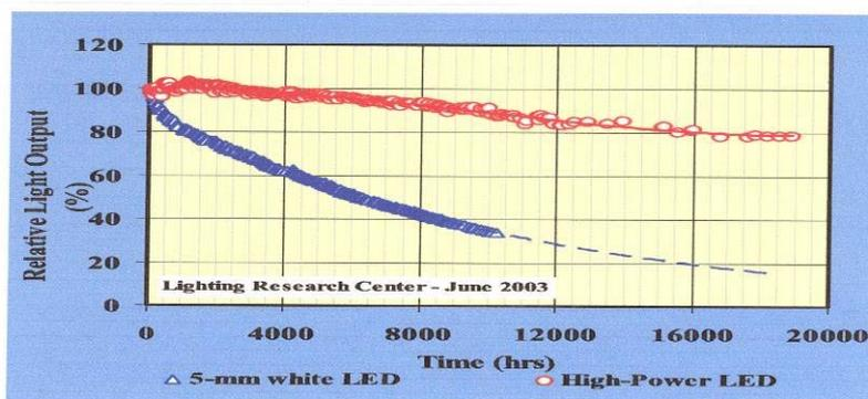
**Figure 10** *Projected Long Term Light Output Degradation for Pulse Drive Condition with The LED On Time Duty Cycle Adjusted to Provide an Average Current  $I_{avg} = 30mA$*
