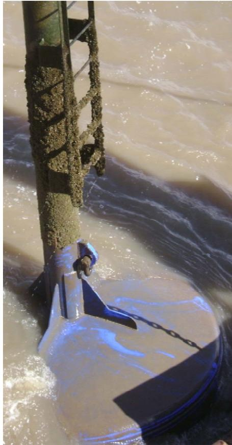
***Figure 1 Spar buoy painted with fluropolymer paint***
