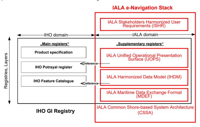
Figure 3 The relationship between the IHO GI Registry and the IALA e-Navigation stack
