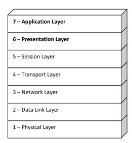
Figure 12 The ISO/OSI Reference Model
