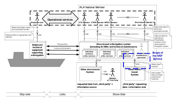
Figure 6 Client-server relationships of the IVEF Service with other shore-based e-Navigation service (see reference [1], Figure 5)
