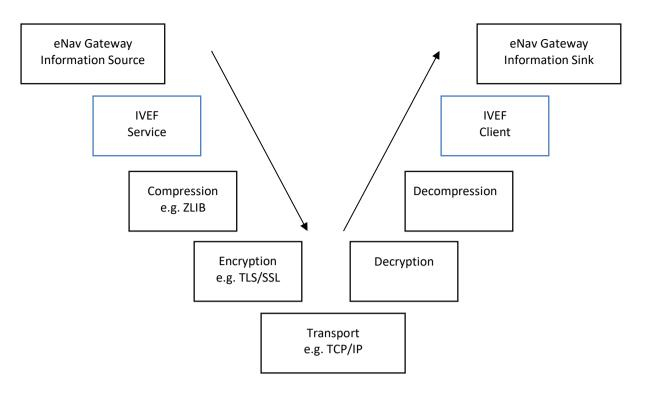
Figure 7 The Communications Stack
