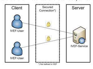
Figure 2 The IVEF Service Client/Server Model
