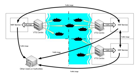
Figure 1 The IVEF Service in operation
