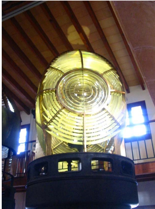
Figure 8 Lower level floor with a mercury bath, rotating machine and revolving optic (Manufactured by Chance Brothers, England) that was installed in Llebeigt Lighthouse from 1910 to 1973. It was transferred from Dragonera Island to Porto Pi Lighthouse Museum by a US helicopter as an underslung load.
