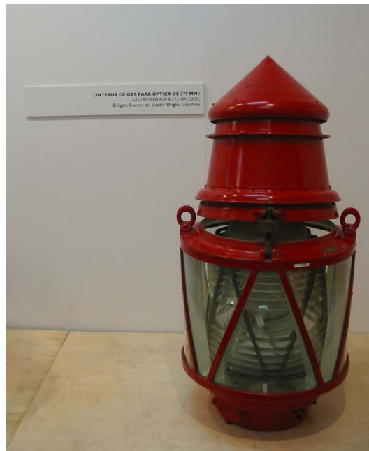
Figure 9 AGA optic 375 mm. Acetylene gas lantern with helical uprights and curved glass. Polished glass drum optic
