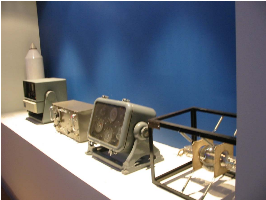
Figure 11 Radioaids. From left to right: 1.- Radar beacon model Sea Watch (Marconi). 2.- User's receiver for the Decca System (Setenil-Cadiz). 3.- Decca Station signal generator (Boal-Asturias). 4.- User's receiver for Decca System (San Juan de Río-Orense) used to check the broadcasts of its three slave stations. 5.- Radio beacon amplification electronic valve (Marconi)
