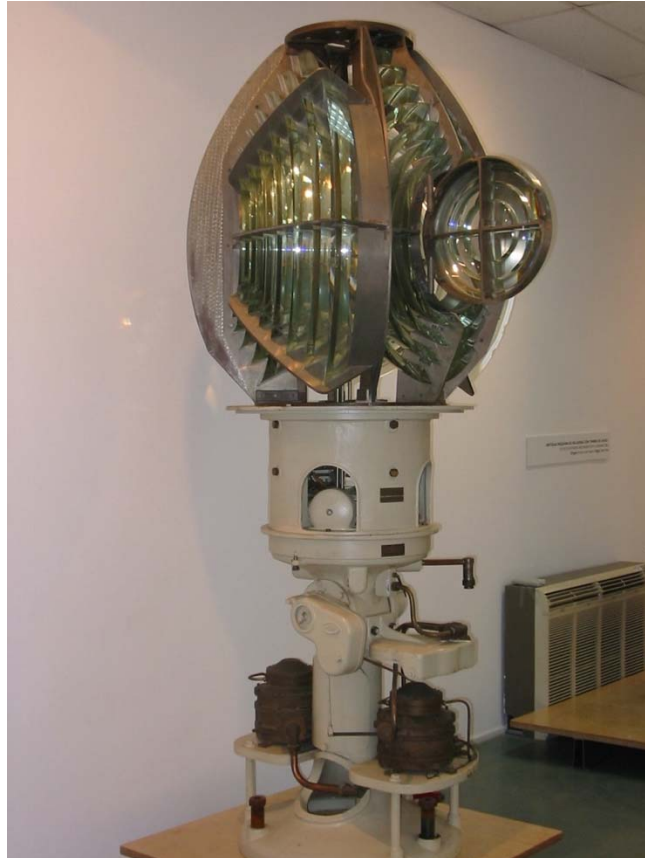
Figure 12 Dalen system acetylene gas apparatus with revolving optic. Dioptric catadioptric optic with 300 mm focal distance lenses and a characteristic group of 2+1 flashes. Tras-130 gas mixers. Manufactured by AGA (Sweden)
