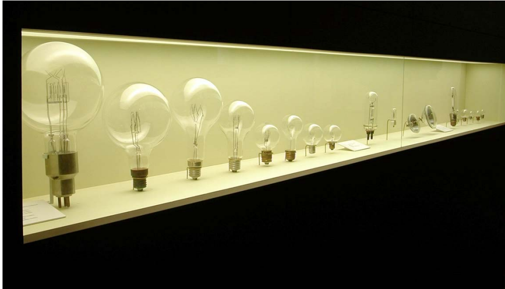
Figure 10 Various types of electric lamps for lighthouses. Selection of some models used in Spanish lighthouses which, because of the characteristics and shape of their filaments, had to be specially made.
