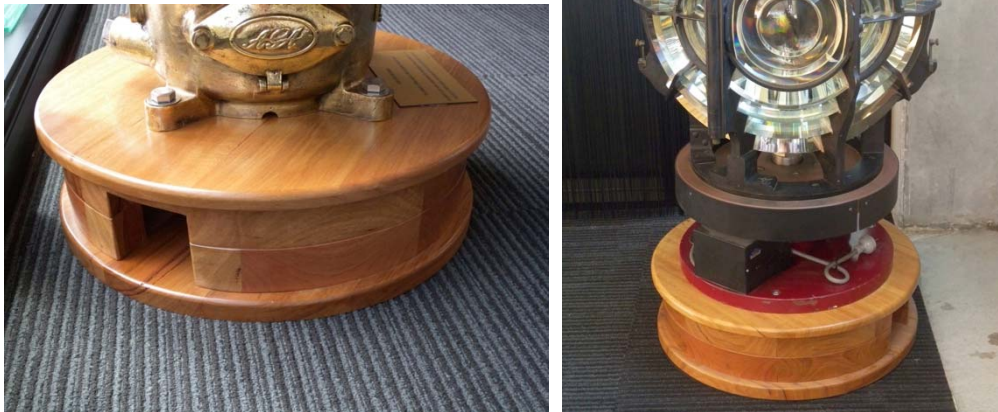
Figure 3 Wooden support bases manufactured to suit specific rotating flashing lenses
