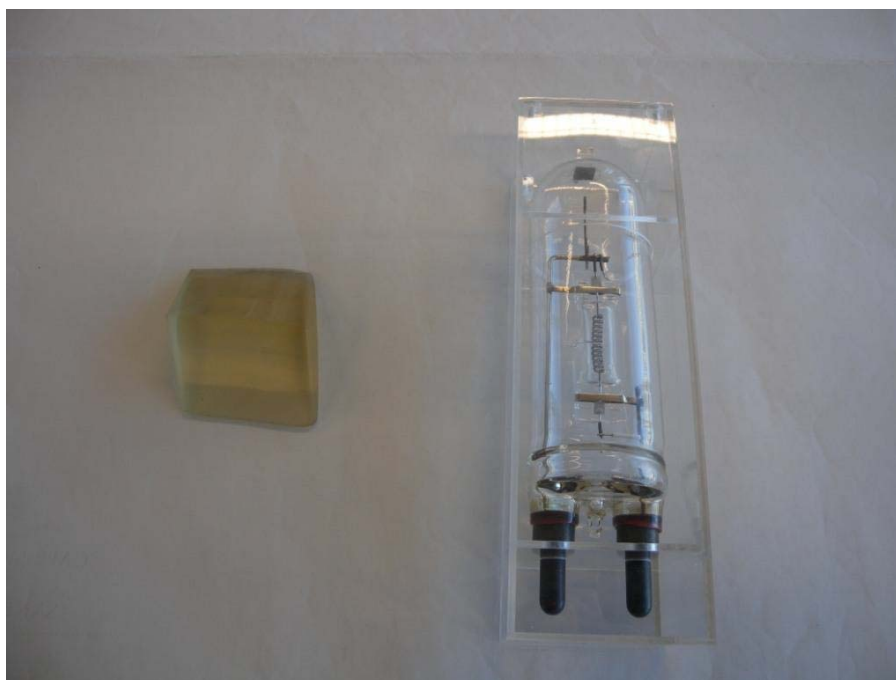
Figure 1 Fresnel glass lens section and 1000W lamp in protective container prepared as props for visitors to handle and inspect.
