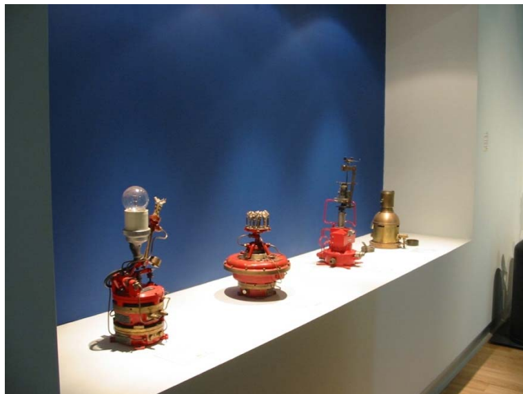
Figure 13 From left to right: 1. - Electric lamp with a Goliath bayonet-type lamp holder with a flashing changer model AGA and lamp acetylene gas reserve. 2. - Flashing bare acetylene gas flame lamp with multiple burners. 3. - Incandescent acetylene gas mantle burner with automatic changer. 4. - Chance 85 mm lamp for a petroleum gas pressure incandescent mantle light installation.
