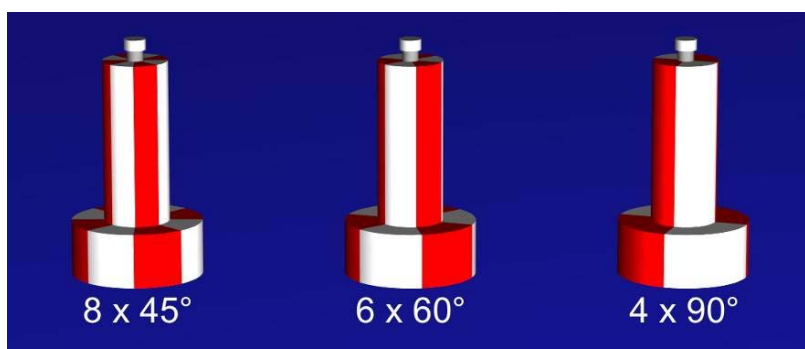
Figure 24 Vertical stripe arrangement on a safe water buoy
